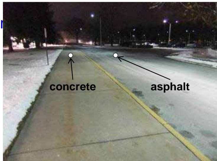
Use spectral radiance of a white diffuser put at "concrete" as spectral radiance of the adaptation field
