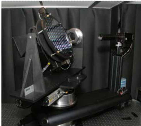
GOSI, an example out-of-plane goniometer
