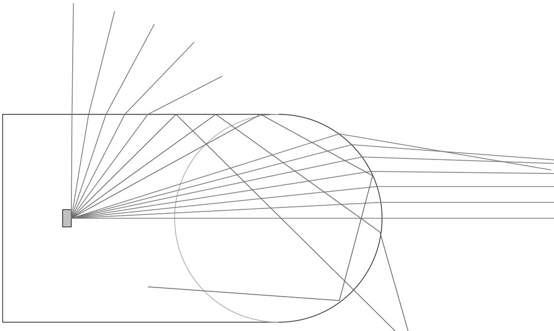
**Figure 1.** A simple ray-trace of a modeled LED package shows that light emerging from a LED can be complex even when the design is simple. Rays through the front lens may be concentrated, or even focused. Rays through the side wall are refracted forward, and rays between these undergo total internal reflection before leaving the device.
