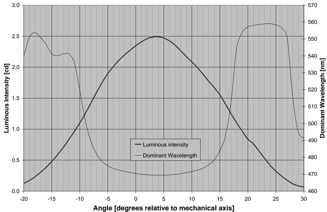
**Figure 2.** Studies of several angular parameters of LEDs can reveal a more complete picture than intensity variations alone. The white LED measured here shows large changes in dominant wavelength with angle, making it potentially unsuitable for some applications.
