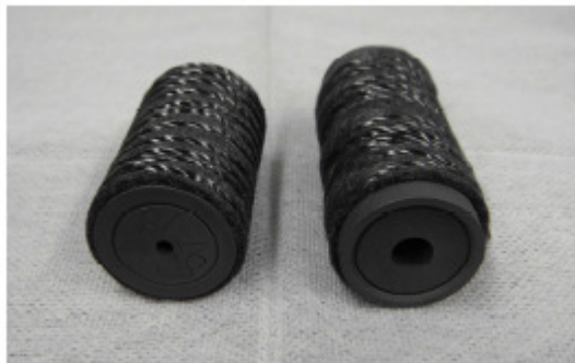
Blackbody cavities, with two aperture sizes and protective sleeves. Photo courtesy Y. Yamada.
