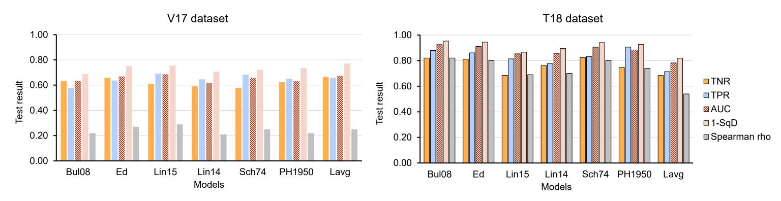
Mean of four diagnostic tests (TNR, TPR, AUC, 1-SqD) for the seven models using individual data sets. A higher mean value indicates a better performance.
