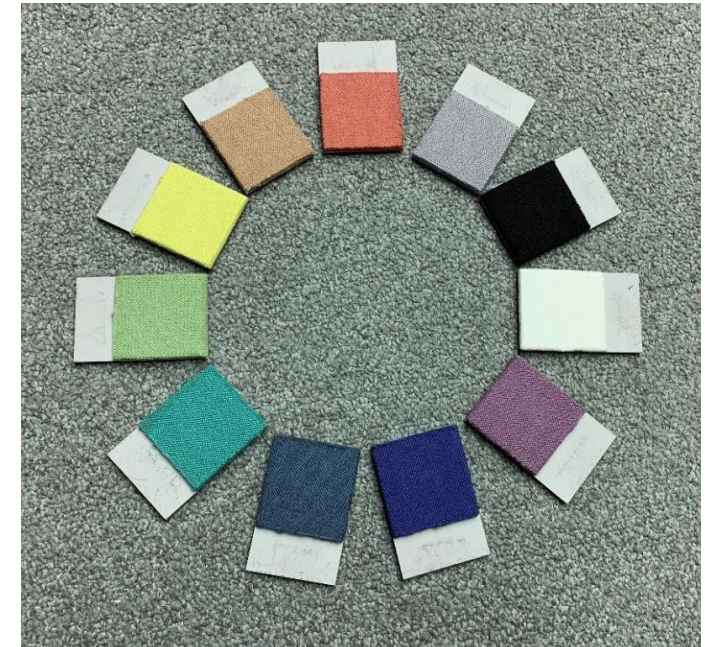
Fig 3. Knitted textile samples in the colors approximating black, white, and nine CIE-recommended color centers.
