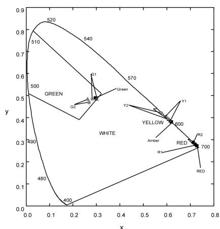
Squares are the locations of filters taken from a wayside signal lights, triangles are the CNLan colors and circles are the colors for the simulation display
