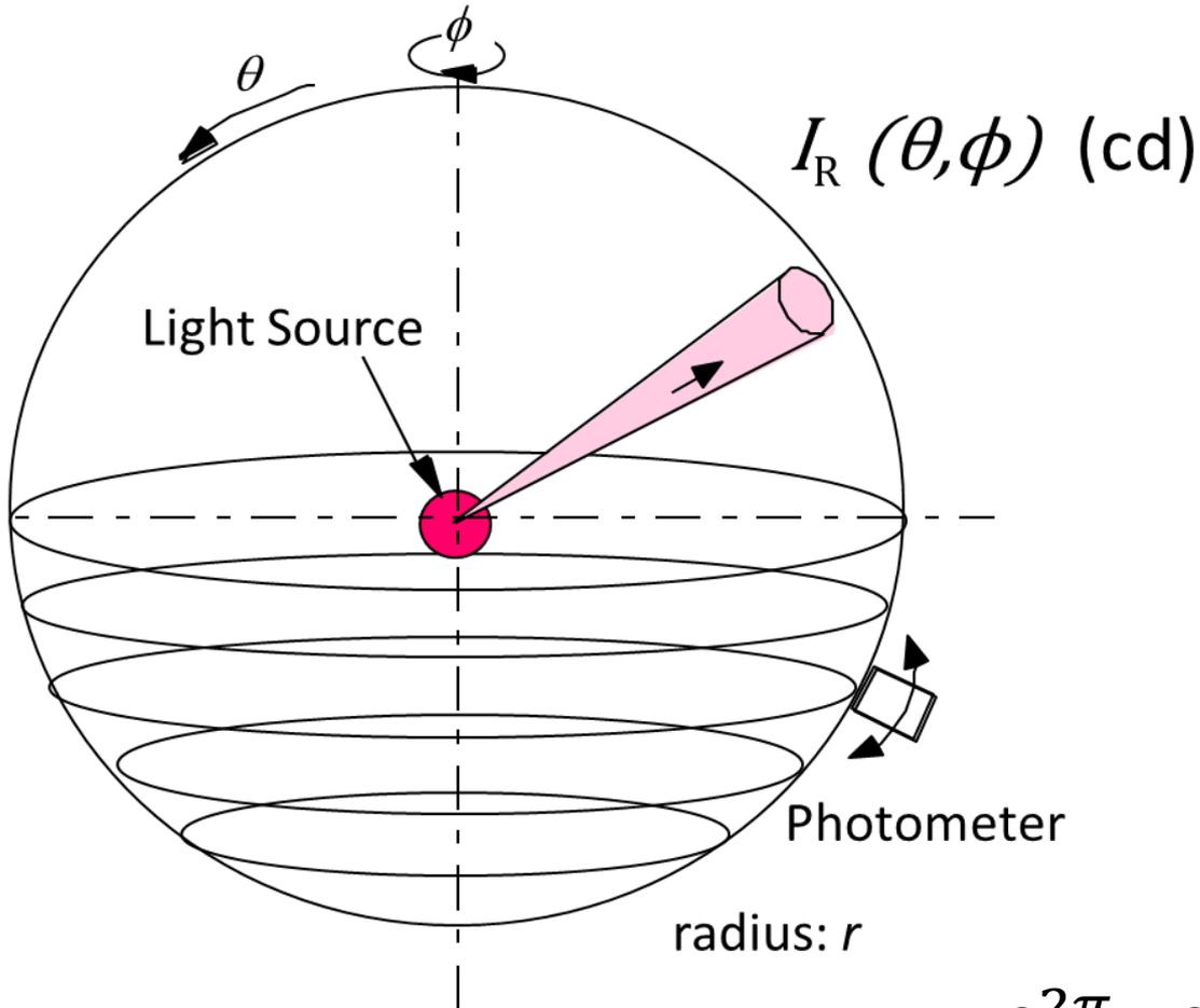
$$\Phi_R = \int_{\phi=0}^{2\pi} \int_{\theta=0}^{\pi} I_R(\theta, \phi) \sin \theta d\theta d\phi$$
