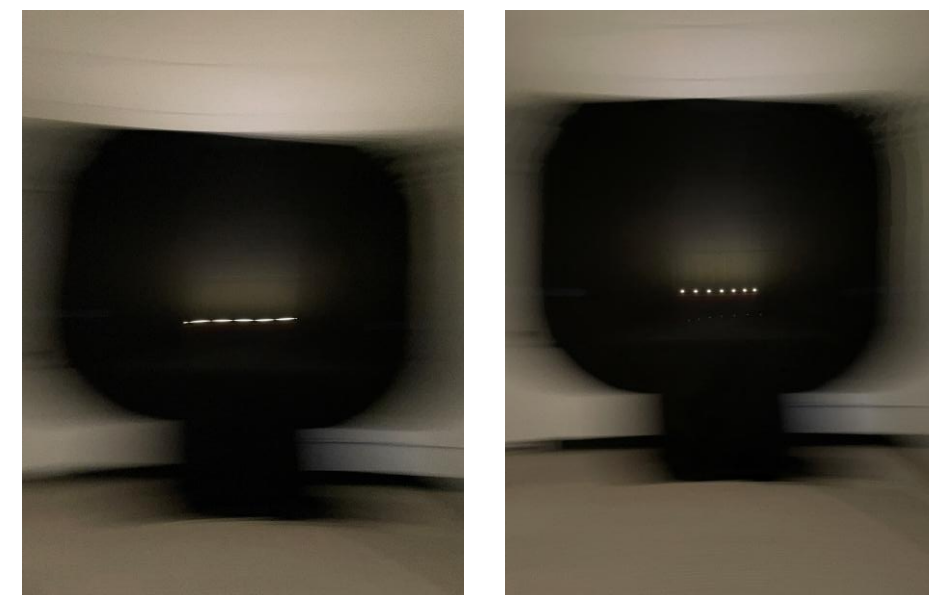
Images of the phantom array effect, sine wave (left) and rectangular wave with 10% duty cycle (right)
